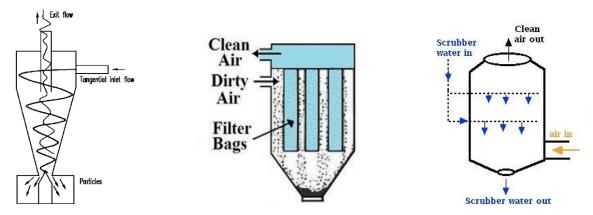
**iv**)Wet scrubbers: These devices trap suspended particles by direct contact with spray of water or other liquid. In a spray tower, an upward flowing airstream is washed by downward sprayed water from a series of nozzle. Spray towers remove 90% of particles with size larger than 8  $\mu$ m. Venturi scrubbers are the most efficient wet scrubbers (Fig).
